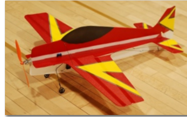
Modern RC foam planes, like the BlingBlingV3 are made with 3mm Depron. This plane is outfitted with the same servos and a similar motor we use in our club planes. Free plans were found on RC Groups.
